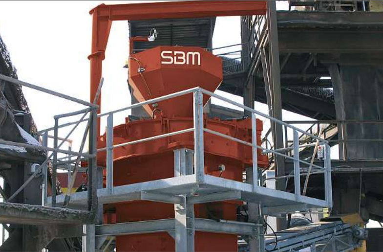
Pic. 1 + 2 SBM vertical impact crusher in operation
