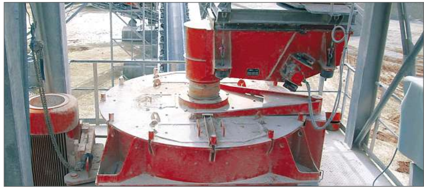
Pic. 1 Multipactor in operation, with vibrating feeder
