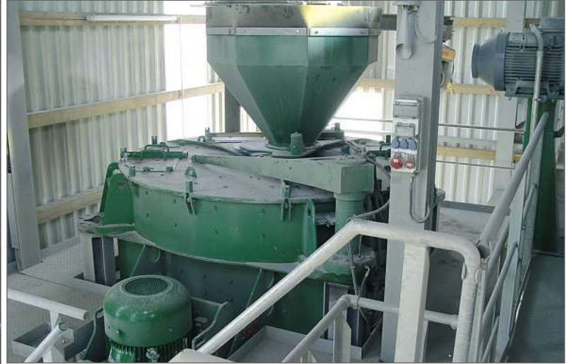
Pic. 1 + 2 SBM vertical impact crusher in operation
