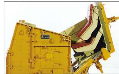
Pic. 3 Impact aprons 1 and 2
