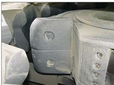
Pic. 2 Rotor with 2 blow bars and impact ring
