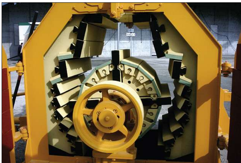
Pic. 1 Crushing chamber of an SMR with wear parts Closed rotor with 4 straight blow bars
